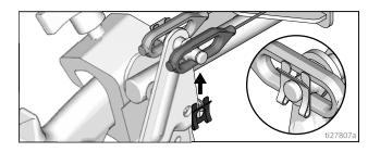
Route cable around unit and up through cable holes behind hose mount.
