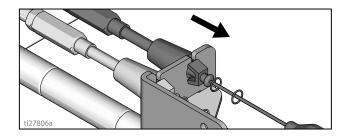
Install cable end onto trigger plate pin and install clip.
