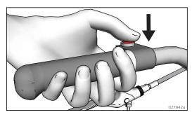
3. Press and release gun trigger control to end measured length. Up to six lengths are viewable.
