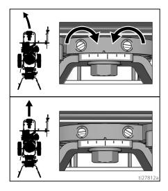
Roll the striper. Repeat steps 2 and 3 until striper rolls straight. Tighten bolt on wheel alignment plate to lock the new wheel setting.
