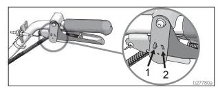
One gun: Disconnect one gun selector plate from trigger.
