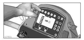
3. Press and release A to end measured length. Up to six lengths are viewable.
