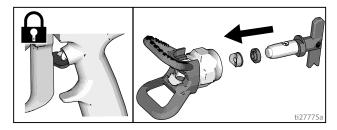
Insert SwitchTip in tip bore and firmly thread assembly onto gun.
