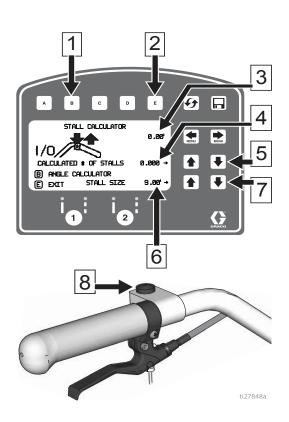
Ref. Description Opens Angle Calculator Menu. See Angle Calculator, page 41. 2 Exits and returns stall size to Layout Mode. Measured distance. Calculated # of stalls. Changing the number of stalls will change the stall size. 5 Adjusts number of stalls. Stall size. Changing stall size changes the calculated # of stalls. 7 Adjusts stall size. Press to start measurement, Press to stop measurement.
