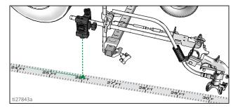
Press and release gun trigger control to complete calibration.
