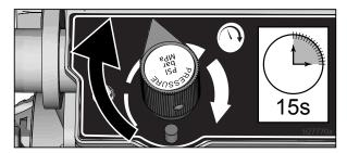
16. Turn pressure down, turn prime valve horizontal. Disengage gun trigger lock.
