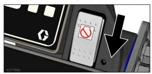
15. Increase pressure control enough to start pump. Allow fluid to circulate for 15 seconds.
