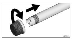
8. Turn prime valve down. Turn pressure control counterclockwise to lowest pressure.
