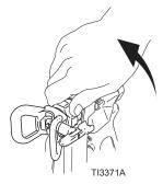
3. Unscrew cap, remove filter. Assemble without filter.
