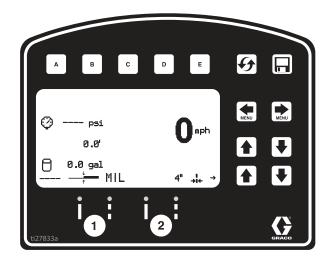
14. Set pump switch to **ON** (pump is now active).
