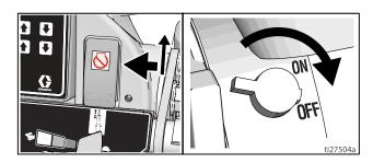
3. Turn pressure control to lowest setting. Trigger all guns to relieve pressure.
