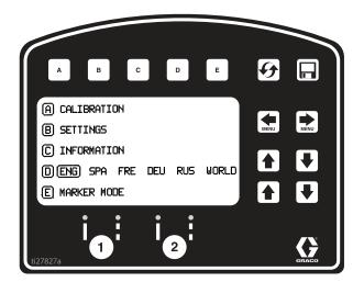
4. Press A for Calibration. Set TRAVEL DIST to 25 ft (7.6m) or longer. Longer distances ensure better accuracy, depending on conditions.
