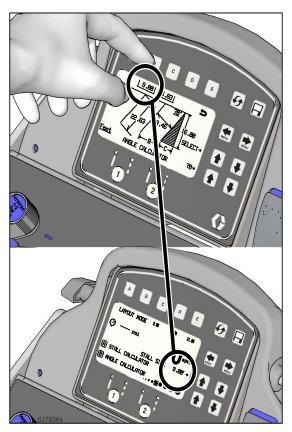
5. Press and release gun trigger control to start marking stall size dots. Press and release gun trigger control to stop marking.
