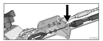
3. Insert plastic cable retainer into cable bracket hole.
