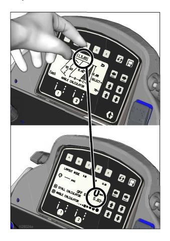
4. Press B to transfer calculated dot spacing distance to Layout Mode. Save this value in favorites if desired.
