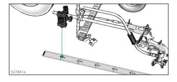
Press and release gun trigger control to start calibration.
