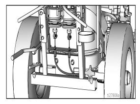
Route cable end loop through rectangular hole in bracket and insert plastic cable retainer into the actuator bracket. Install cable end onto actuator rod and install pin.
