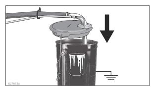
20. Trigger all guns again into a flushing fluid pail until paint appears. Assemble tips and guards.
