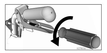
4. Continue adjusting screw in handle until timing of spray icon and fluid spray are synchronized. Adjustment of the gun cables might be necessary.
