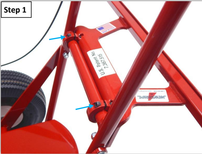
Step 1: Mount the rail to the handle using the provided hex wrench.
