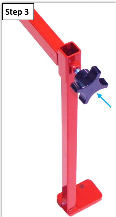
Step 3: Install the downtube in the receiver at the right side of the rail. The plate on the bottom of the downtube should have the bolt hole toward the front of the machine. Adjust the down tube so that the plate is about 4" off the ground and then tighten the star knob.
