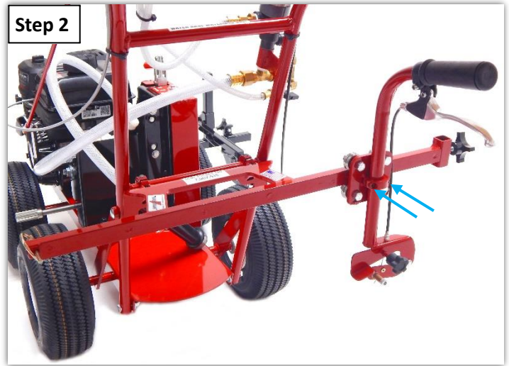
Step 2: Install the gun mount assembly into the collar carriage using the provided hex wrench. Tighten the screws just enough to hold it in place.
