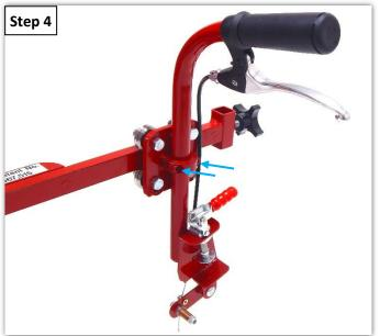
**Step 4:** Install the gun mount assembly into the collar carriage using the provided hex wrench. Tighten the screws just enough to hold it in place.
