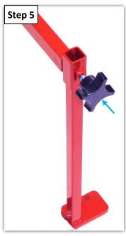
**Step 5:** Install the downtube in the receiver at the right side of the rail. The plate on the bottom of the downtube should have the bolt hole toward the front of the machine. Adjust the down tube so that the plate is about 4" off the ground and then tighten the star knob.
