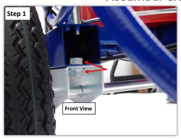
**Step 1:** Remove the two rear axle bolts and nuts on the right side of the machine. Discard the nuts and the rear axle bolt only. Note: Keep the front axle bolt for reassembly.
