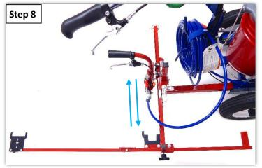
**Step 8:** Roll the carriage back and forth on the rail to make sure that there is no interference with the paint hose. Open the strap holding the coiled paint hose and adjust it if necessary.
