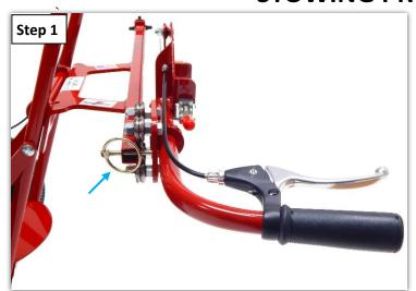
Step 1: Remove the spray gun from the HashMark Master<sup>TM</sup> and place it back into the gun mount of the machine. Remove the lynchpin and roll the carriage and gun mount assembly off of the rail. Rotate the carriage and gun mount assembly 90 degrees, and then roll it back onto the rail. Install the lynchpin through the rail and into the hole in the carriage plate, as shown.
