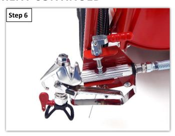
**Step 6:** Remove the spray gun from the gun mount of the machine, and place it in the gun mount of the HashMark Master<sup>TM</sup>. Secure it in the gun mount with the gun mount clamp.
