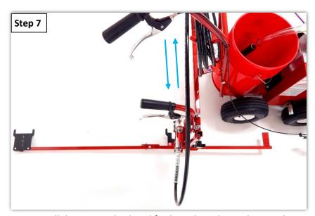
**Step 7:** Roll the carriage back and forth on the rail to make sure that there is no interference with the paint hose. Open the strap holding the coiled paint hose and adjust it if necessary.
