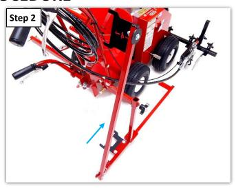
**Step 2:** Rotate the rear line guide tube upward, and allow it to rest against the front line guide tube, out of the way as shown.
