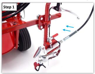
**Step 1:** Loosen the screws on the carrier and then raise or lower the gun mount assembly until a 4" wide line is made, when you spray.
