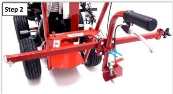
**Step 2:** Install the gun mount assembly into the collar carriage using the provided hex wrench. Tighten the screws just enough to hold it in place.
