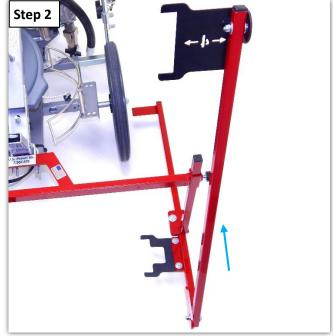
**Step 2:** Rotate the rear line guide tube upward, and allow it to rest against the front line guide tube, out of the way as shown.
