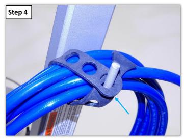
**Step 4:** Wrap the hose with the provided strap so that the hose does not contact the rail as the carriage moves.
