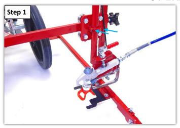
**Step 1:** Loosen the screws on the carrier and then raise or lower the gun mount assembly until a 4" wide line is made, when you spray.
