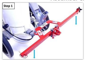
**Step 1:** Fold the machine handle forward. Mount the rail just below the folded top portion of the handle, with the provided U-Bolts, as shown. Lightly snug the nuts to hold it in place. Measure the distance of both ends of the rail to the ground, on a flat surface to level the rail, and then fully tighten the nuts.
