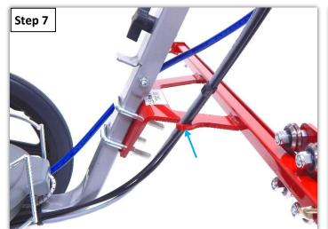
**Step 7:** Place the cables of the machine in the hook of the rail plate, to keep them from getting damaged from the carriage during operation.
