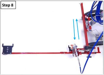
**Step 8:** Roll the carriage back and forth on the rail to make sure that there is no interference with the paint hose. Open the strap holding the coiled paint hose and adjust it if necessary.
