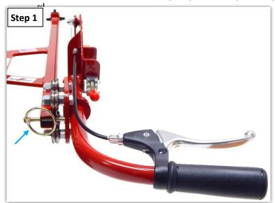
Step 1: Remove the spray gun from the HashMark Master<sup>™</sup> and place it back into the gun mount of the machine. Remove the lynchpin and roll the carriage and gun mount assembly off of the rail. Rotate the carriage and gun mount assembly 90 degrees, and then roll it back onto the rail. Install the lynchpin through the rail and into the hole in the carriage plate, as shown.
