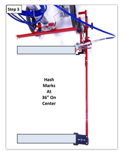
**Step 3:** Position the machine with the cutout of the rear line guide plate, centered over the goal line and the center of the spray tip at the left edge of the cutout of the center line guide plate. In a continuous motion, squeeze the spray lever and roll the carriage along the rail until it makes contact with the lynchpin. This will result in a 24" hash mark line.
