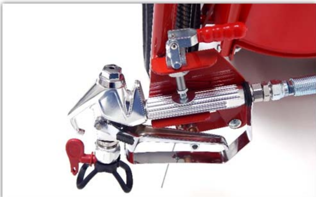
Step 4: Clamp the gun into the gun mount.
