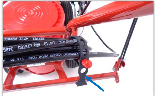
Step 3: Lightly wrap the hose to the hanger using the provided strap.
