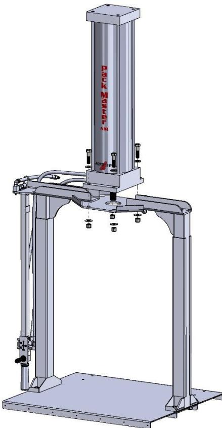
5. Insure that the jam nut is spun all the way up on the threaded portion of the air cylinder rod by hand. Thread the ram plate onto the air cylinder rod until it is snug. Spin the jam nut back down against the ram plate and then tighten it.
