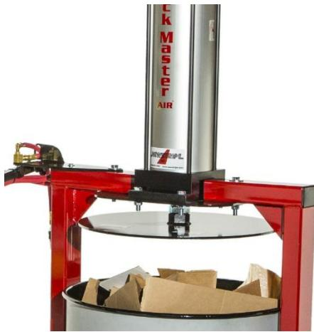
2. Lift the safety control arm to a horizontal position, against the stop on the unit. This assures that the safety valve plunger is fully depressed.
