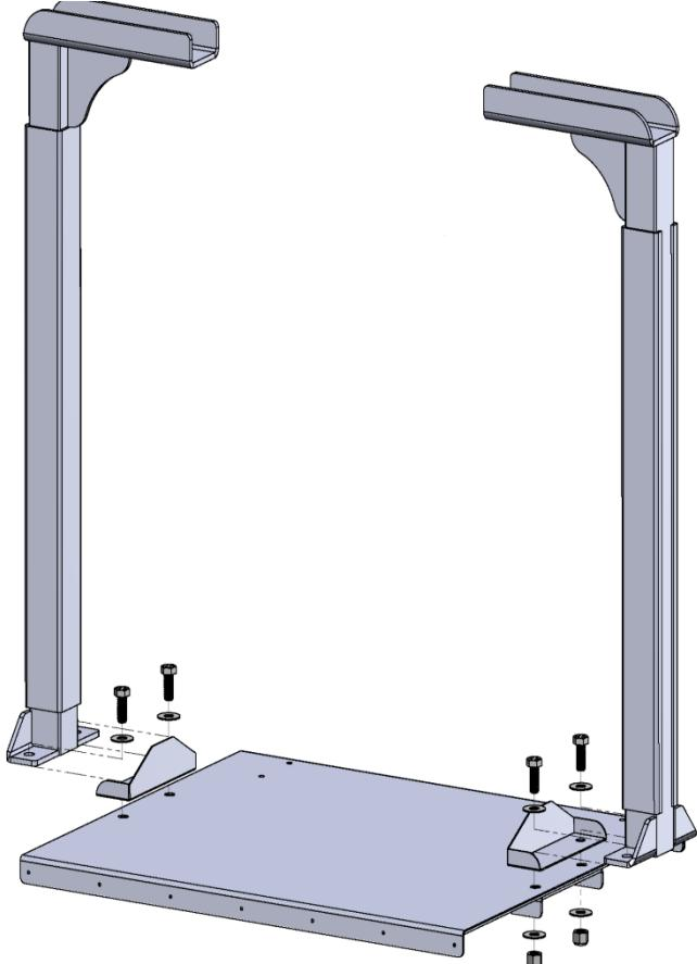
2. Install the control arm and the cylinder plate to the two uprights using (1)  $\frac{1}{2}$ " x 1  $\frac{1}{2}$ " long bolt, (2)  $\frac{1}{2}$ " washers, and (1) locking nut, on the right side, and (1)  $\frac{1}{2}$ " x 2" long bolt, (2)  $\frac{1}{2}$ " washers, and (1) locking nut on the left side, with the bracket.
