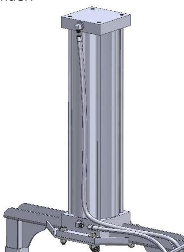
6. Connect the PackMaster to an air supply source with a maximum pressure of 150 psi.
