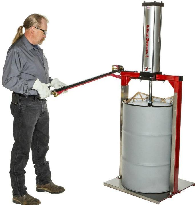
3. Move the ram control valve lever toward the handle end, (backwards) to lower the ram plate. Release the ram control valve lever, and the ram plate will stop. Move the ram control valve lever toward the unit (forward) to raise the ram.
