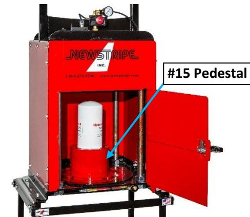
4. If desired, place the splash guard over the pedestal to help contain splash during the crushing process.
