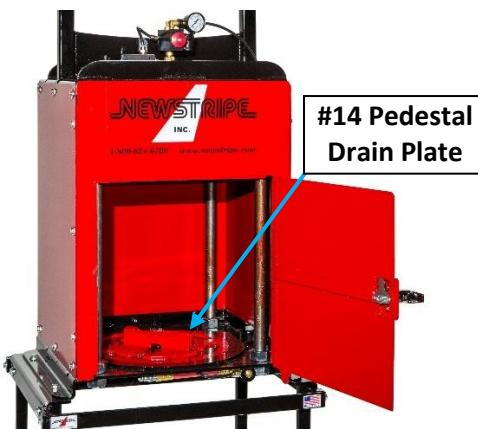
3. Set the pedestal over the pedestal drain plate in the center recess of the alignment ring.
