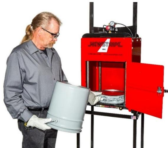
2. Push the button on the cycle valve on the top of the unit. The air pressure reading on the gauge will climb until it reaches the factory setting of 85 psi. The cycle button will then pop back out, and air will vent as the ram plate retracts. Once the pressure begins to drop, the door may be opened, and the crushed container or filter may be removed.
