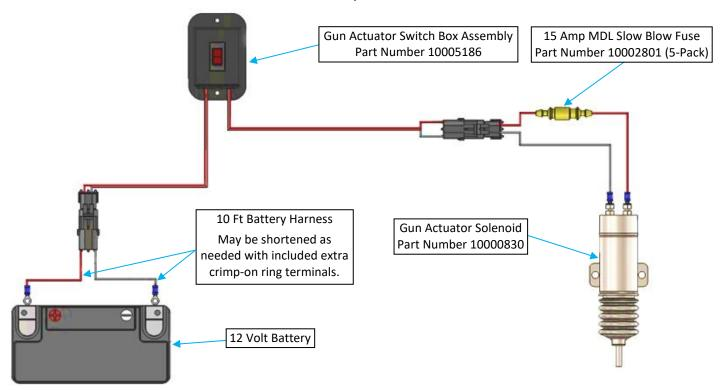
WARNING: The Gun Actuator Solenoid must never be energized if the gun trigger is locked. The solenoid must always be able to retract fully when energized or the solenoid will burn out in less than one minute. The circuit uses a 15 Amp MDL <u>SLOW BLOW</u> Glass Fuse. DO NOT USE A HIGHER AMP FUSE or you may cause damage to your system. Do not operate the solenoid without the vehicle engine running or you may deplete the charge on the battery and damage the solenoid.
