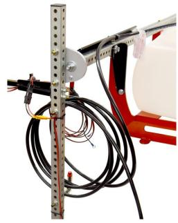
5. Remove the gun mount from the padded envelope and slide it down onto the spray head upright post. Secure it with the receiver tube at about 3" up from the post base by tightening the pinch bolt. Clamp the spray gun in the gun mount as shown, with the actuator bar under the gun trigger. If the gun trigger will not move, release the trigger lock by pushing the lock in from the right side (inside) of the gun.
