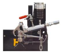
6. Position the pointer so that the dangle marker will be at the inside of the painted line and then secure it with the star knob. For example, if you are painting a 4" line, the dangle marker should be 2" in from the center of the spray nozzle. Some fine tuning may be needed, so we recommend practicing with water to achieve the desired results before painting. Make sure the static grounding chain hanging from the bottom of the vertical boom rail contacts the ground.
