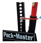
2) Swing the lower lever to the "DOWN" position first, and then the upper lever to the "DOWN" position.
