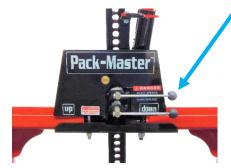
3) Disengage the <u>handle lock</u> and then begin pumping the jack handle up and down.
