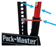
4) To retract the compactor plate, while applying slight downward pressure on jack handle, swing upper lever to "UP" position, then the lower lever. This removes pressure on the pin and will extend the life of the jacking pins.
