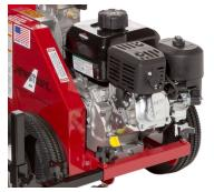
Smooth and Economical: The 127 cc Briggs and Stratton or optional Honda GX120 engines both feature an OHV design for fuel economy and smooth operation and the included oil alert won't let you damage the engine from low oil. Four 10" pneumatic tires make for easy rolling.
