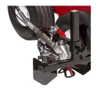
Versatile: A quick release clamp allows you to remove the spray gun to paint stencils, curbs, and hard to reach areas with a 25 foot length hose. An optional HashMark™ Master II is also available to easily and quickly create hash marks on athletic fields.
