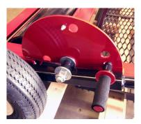
No Tools Required: All adjustments on the Dirt Doctor Jr.™ can be made super fast and require No Tools! You can easily fine-tune the reversible harrow teeth, pulverizer bar, transport wheels and optional finishing broom or drag mat to give your infield the perfect playing surface.
