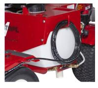
**25 Gallon Tank:** The large 25 gallon tank allows for more time painting and less time refilling your supply. A single tank provides enough coverage to paint up to 5 soccer fields or 2.5 football fields.
