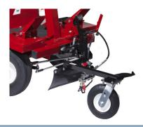
Floating Spray Head: The floating spray head allows for even lines on even the most bumpy of fields. Equipped with a pneumatic wheel that leads the spray gun, the floating head keeps a consistent spray pattern over any dips and bumps that a field may have.
