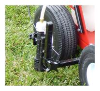
Removable Spray Gun The FieldLiner 3<sup>™</sup> removable in line gun sprays 2"- 6" wide lines with a five hose for painting stencils and hard to reach areas. There is an in gun cleanable strainer for easy cleaning.
