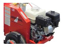
No More Pushing: The 4600 SP Self Propelled striper is in a class of its own. Powered by a Honda GX120 with oil alert for long life and dependability. Ideal for athletic fields or large jobs when pushing is not ideal. Get more done with less fatigue. The simple friction drives pulls the striper even over uneven surfaces.
