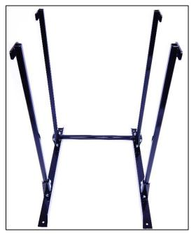
4) Install the left and right upper support rails to the support legs using four 1" bolts with eight flat washers, and four nylock hex nuts. Install the rails so that the slotted hole on the top of each rail is to the rear and so that the side of each rail is to the outside of the leg tabs.
