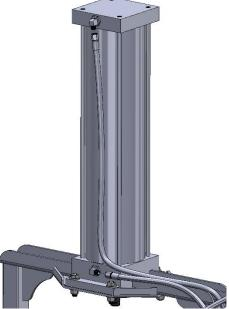
8. Check that the jam nut is spun all the way up on the air cylinder rod threads by hand. Thread the ram plate onto the air cylinder rod until it is snug. Spin the jam nut back down against the ram plate and tighten it.
