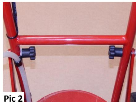
5. Insert the spray head support arm into the receiver tube on right side of the chassis until it stops and then secure it with one large star knob.
