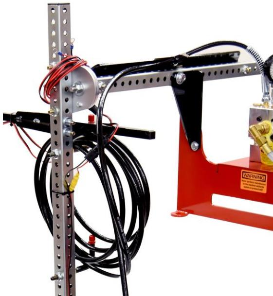
5. Remove the gun mount from the padded envelope and slide it down onto the spray head upright post. Secure it with the receiver tube at about 3" up from the post base by tightening the pinch bolt. Clamp the spray gun in the gun mount as shown, with the actuator bar under the gun trigger. If the gun trigger will not move, release the trigger lock by pushing the lock in from the right side (inside) of the gun.
