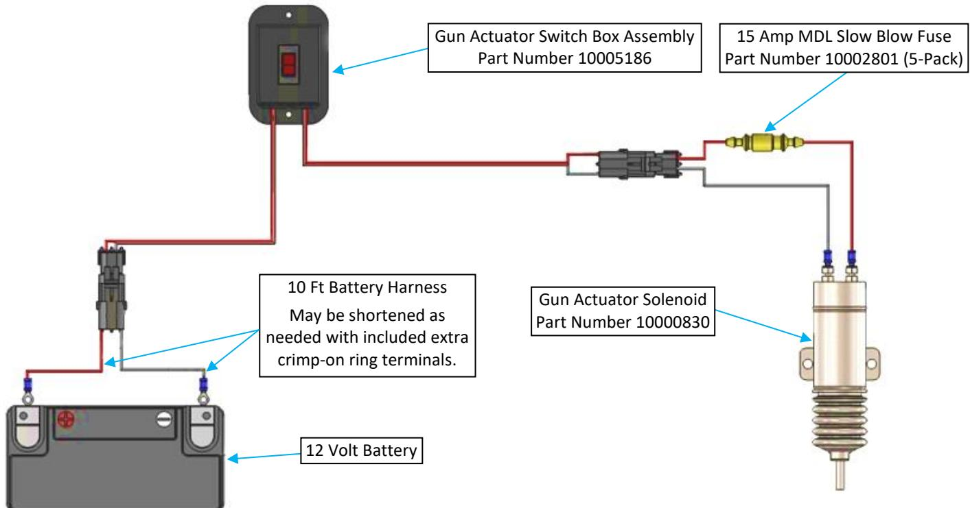
**WARNING:** The Gun Actuator Solenoid must never be energized if the gun trigger is locked. The solenoid must always be able to retract fully when energized or the solenoid will burn out in less than one minute. The circuit uses a 15 Amp MDL SLOW BLOW Glass Fuse. DO NOT USE A HIGHER AMP FUSE or you may cause damage to your system. Do not operate the solenoid without the vehicle engine running or you may deplete the charge on the battery and damage the solenoid.
