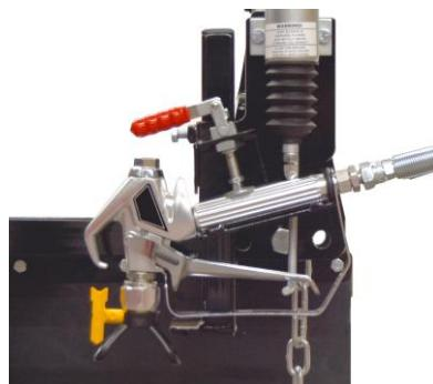
6. Position the pointer so that the dangle marker will be at the inside of the painted line and then secure it with the star knob. For example, if you are painting a 4" line, the dangle marker should be 2" in from the center of the spray nozzle. Some fine tuning may be needed, so we recommend practicing with water to achieve the desired results before painting. Make sure the static grounding chain hanging from the bottom of the vertical boom rail contacts the ground.
